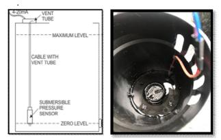
Figure 7. Installation of water level sensor in MHS
